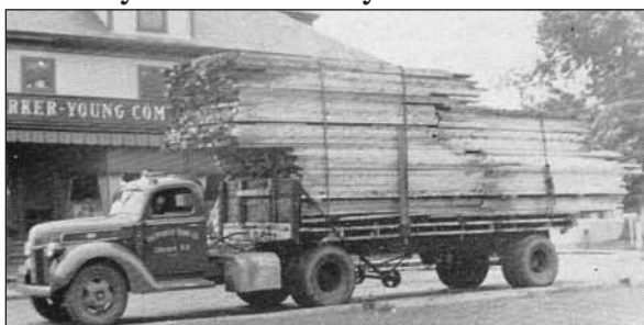
P. Y. CO. LUMBER TRAILER with a load of 14,000 F.B.M. Dimension Spruce
